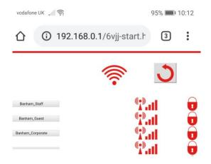
• Select the router that you wish the alarm panel to connect to, enter the router password and then select the 'tick' button
